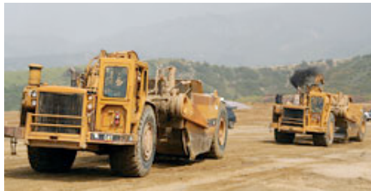
Clearly Different. Visible fumes spew from the scraper on the right, which has original 1980 engine. The scraper on the left was repowered last year. CARB issued letter (below) to 79,000 contractors.
